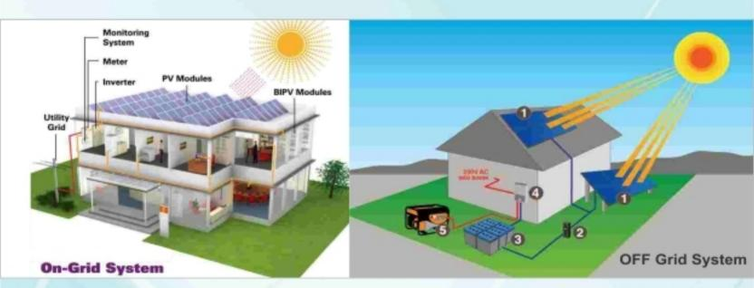
OFF GRID SYSTEM: - In this model the energy produced by the PV panels is used to charge the battery to provide power in the absence of grid power and also to minimise the energy usage from the utility grid. This system is ideal for locations which experience frequent power failure and need autonomy. Capacity 1-5 Kw. Key Components: OFF grid Inverter, PV Panels, Batteries.
